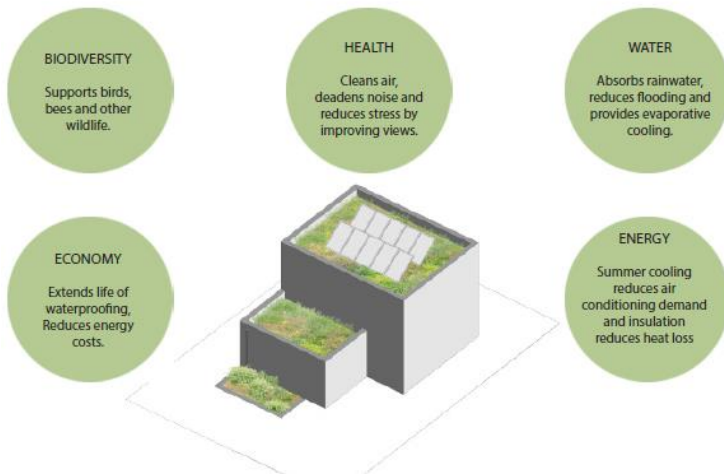
Figure 2. Green roofs for example provide many benefits which enable developers to reach GSF targets
